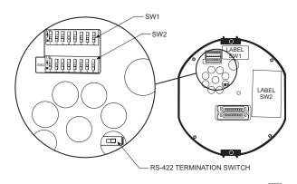
a. Set the DIP switches for SW1 and SW2 on the bottom of the dome drive for the appropriate receiver address. Refer to the labels on the dome drive or Tables C through E in the Appendix in the back of this manual.
